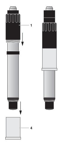
**3** Insert the sensor with the mounted retaining ring in the sleeve (4) and fix it using the swivel nut (1).
