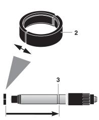
Carefully widen the retaining ring (2) at the ring opening and slide it over the sensor shaft up to the groove (3).
